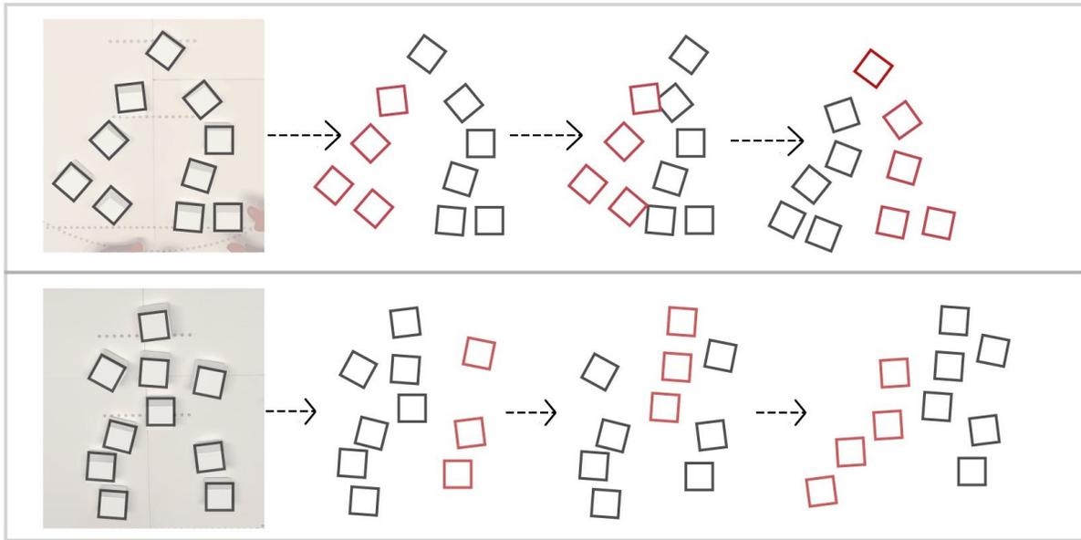
**Figure 1: Two user-defined patterns of swarm robot co-speech gestures corresponding to the word "run." Each pattern includes multiple phases, with red squares indicating the robots that have moved relative to the previous phase.**
