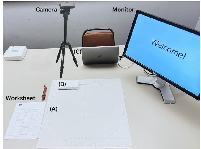
**Figure 2:** Setup for the elicitation study. Participants sat in front of a tracking mat (A) and manually manipulated 10 Toio robots (B). Audio for single-word speech instances was projected from a laptop near the mat (C).
