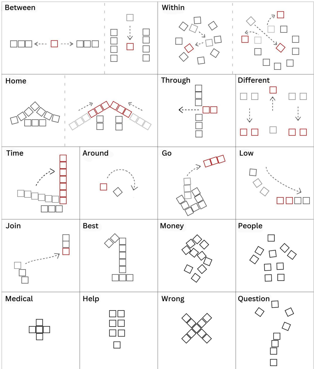
Figure 6: Co-speech gestures for referent words with high agreement scores. For some referent words, multiple co-speech gesture designs are shown, separated by dotted lines. In each design, red squares indicate the robots that have moved from their initial positions. Designs without red squares represent the final formation of the swarm robots after their movements from any previous positions.
